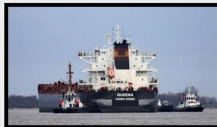
The “Kamsarmax” bulk carrier “**Queena**” operated by the Sincere Navigation Group – Taiwan. Built in 2016 with a deadweight tonnage of 82082 tons, and a max LOA of 229m, and beam of 53m.
