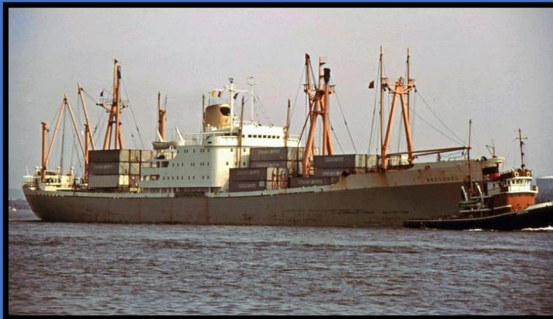
The fine looking 1963 built, CMB cargo liner "**Breughel**" an early participant in the Dart Containerline service to the USA. A good example of ex cargo ships being used for containers during the early 1970s before full containerization became the norm. The ship was eventually sold to Far East interests, ending up as the "**Tamaki**" prior to being sent for
