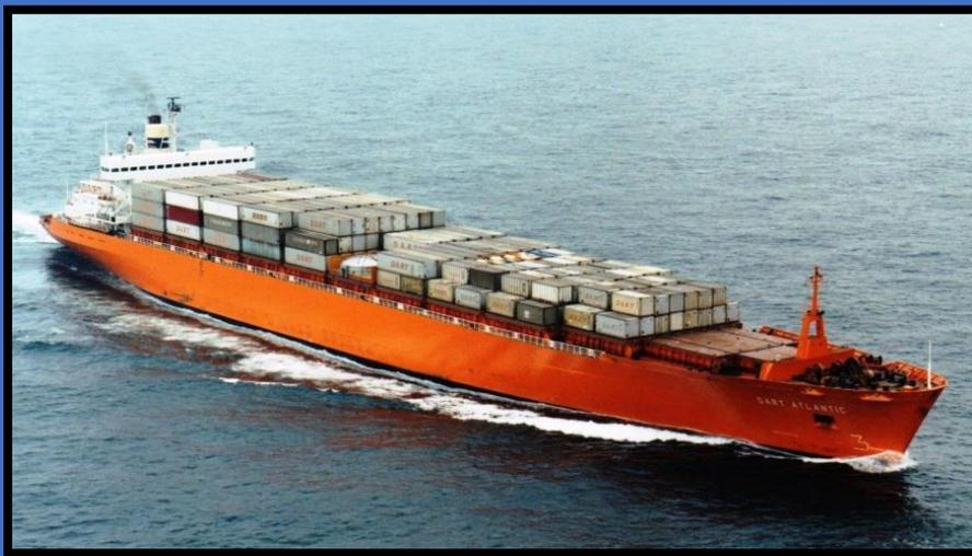
Built in 1971 by Swan Hunter and Tyne Shipbuilders. Grt 31036. Fitted with Sulzer @SA 10 Cylinder Diesel developing 29,000 BHP giving a service speed of 21 knots. With the absorption of **Bristol City Line** into **Bibby Line** the vessel was employed on the **Dart Containerline Service** to North America. In 1986 her name was changed to "**Canmar Ambassador**", she finally met her demise at Alang in 1995.
