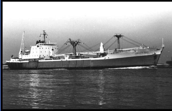
The very streamlined vessel "**MV Toronto City**" built by Doxford shipbuilders, Sunderland, in 1966. Grt 7643. Fitted with 6 Cylinder Sulzer 2SA diesel engine developing 9600 BHP and giving a service speed of 17 knots. This ship changed ownership to Bibby Bulk Carriers Ltd. when the take-over took place during 1971. However, her tenure was to be short lived, because in 1972 she was sold, her name being changed to **Ilkon Polly** and owner to Brandts Sg Liberia Ltd. There then followed, several
