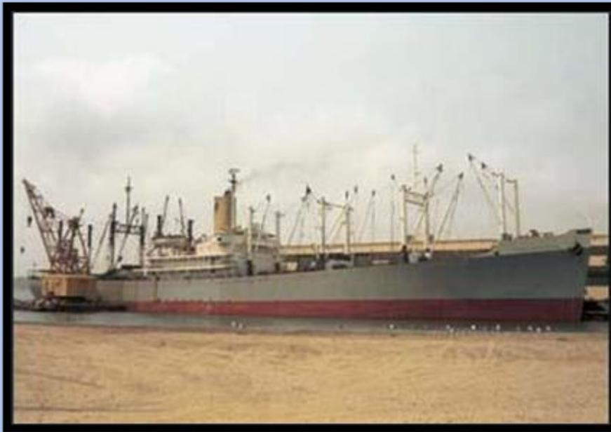
Isthmian Steamship Company "C3" Freighter "**SS Steel Executive**" 8019 GRT, 2 x General Electric Turbines, Speed 18 knots. Built 1945 and joined Isthmian fleet 1947. Sent to demolition at Kaohsiung, Taiwan 1973
