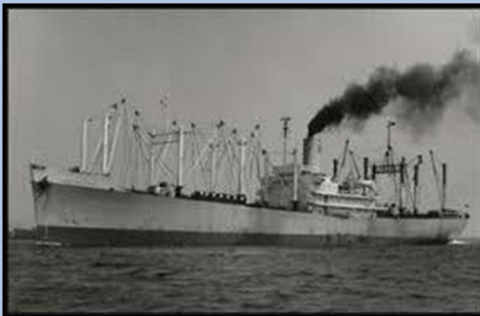
Isthmian's "C3" Freighter "**SS Steel Seafarer**" 7948 GRT, Built 1945. 2 x Westinghouse Electric Steam Turbines with a service speed of about 18 knots. Entered service with Isthmian during 1947 and was sold for demolition in Taiwan during 1973
