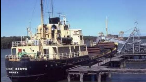
**MV. Stephen Brown**, captured at a coal loading jetty. Note the single coal-loading chute arrangement, meaning the vessel was required to warp along the quay to facilitate loading.
