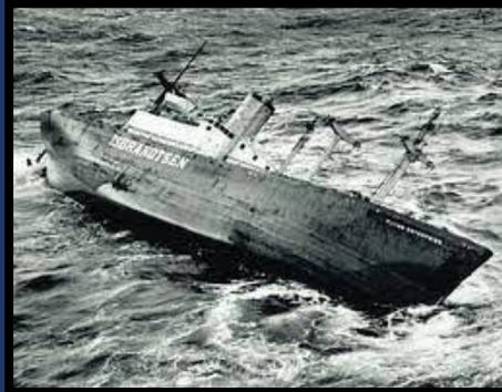
The “**Flying Enterprise**” listing heavily due to the shifting of deadweight cargo
