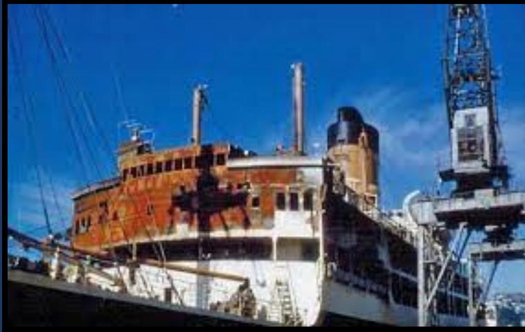
The fire damaged and charred accommodation and Bridge area of the “**TSS Gothic**”, which surely testifies to the ferocity of the inferno.
