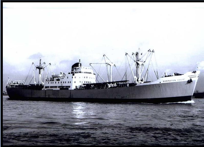
The fine looking **"Dorrington Court"** built in 1957 by Short Bros Ltd., Sunderland, for the Court Line. 6233 GRT, 10,668 DWT. A 4 Cyl B&W diesel engine, giving a service speed of 12 knots.
